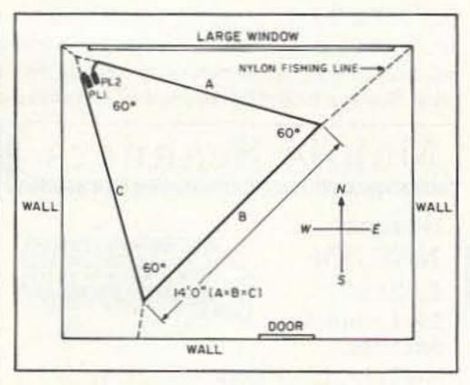
Figure 2. Installation of the Loop.
